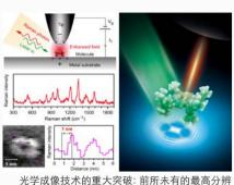
单分子光学成像与化学识别, 分辨率高达 0.5nm Breakthrough in optical microscopy-Realization of unprecedented high-resolution single-molecule Raman microscopy, the spatial resolution reaches 0.5 nm.
